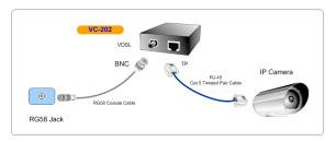
Figure 3-4: Connecting Standalone IP device
